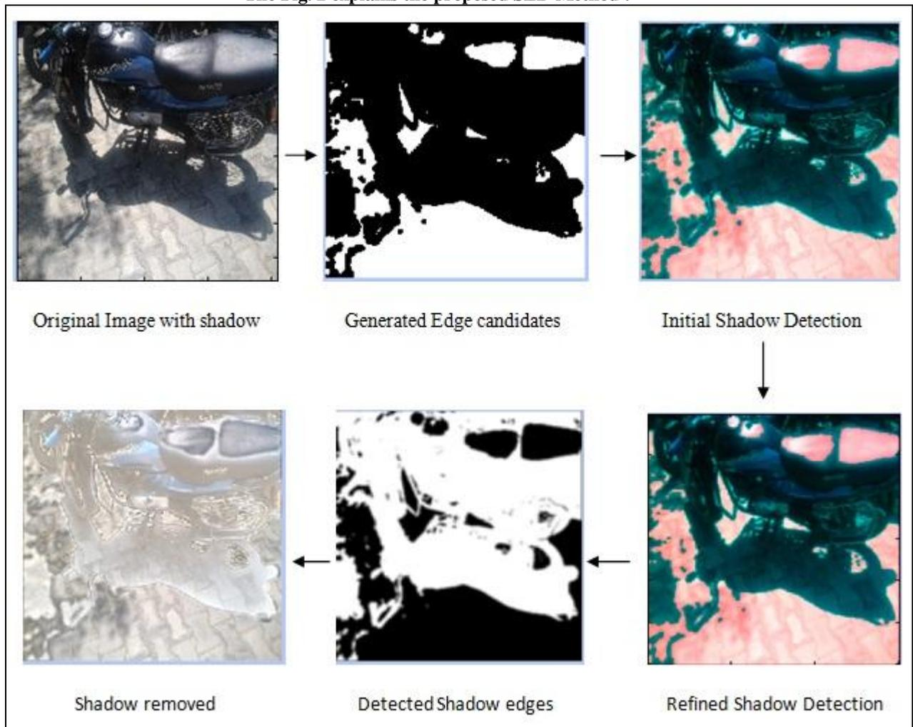
**Fig. 2** Pictorial representation of proposed SED Method
