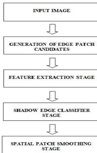
**Fig. 1** Flowchart of proposed methodology for shadow removal which is based on Strong Edge Detection (SED) method.
